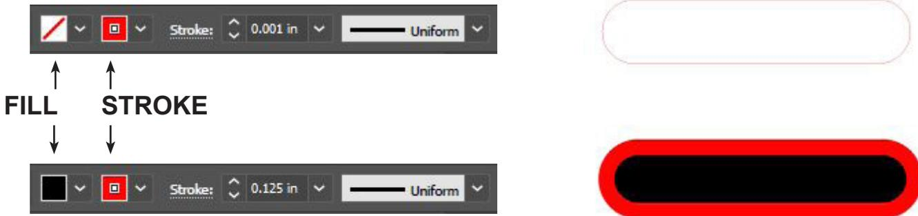
The vector in this example has a **black** fill and a stroke color of **RGB red**. The vector's stroke weight is greater than .001 in, so it is not a cut line.
