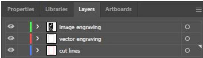
Ideal layer setup. This is how files should come to the lab.
