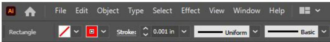
Vector lines can also be used for engraving. Any vector line with a stroke weight greater than **0.001 in** will register in the driver as a line to be engraved. Let's look at the example below:
