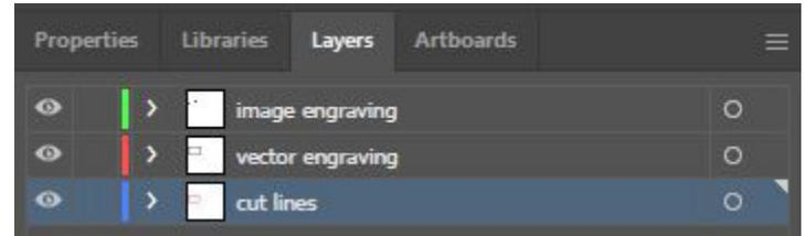
When running a file with multiple operations, it is strongly recommended that each element is set to its own layer. While the laser can run vector and raster settings at the same time, having these operations on individual layers gives users greater control in the lasering process.
